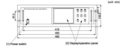
Figure 2-1A: Model 7500ZA Front Panel
